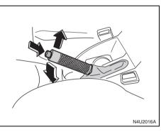
The parking brake lever is located between the bucket seats.
